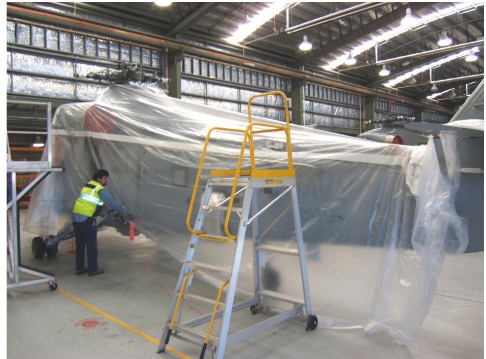
Making the Pattern – Under-Raps specialist measures up the Sea Sprite
