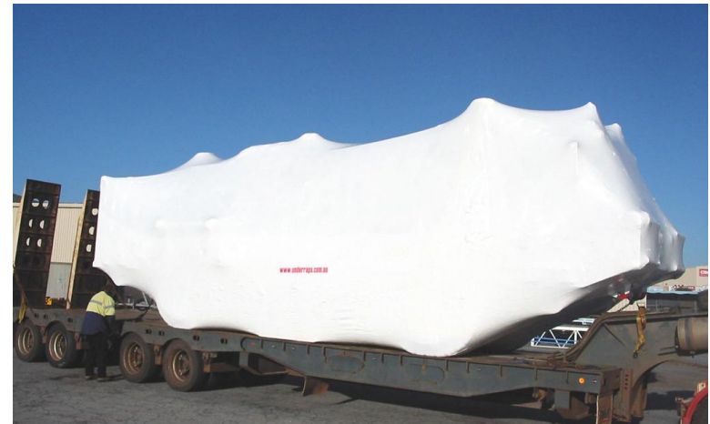
Outer Layer Fitted –Shrunk Tight
