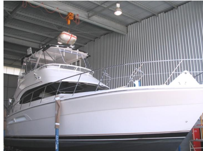
Cover hoisted above boat for unfurling.
