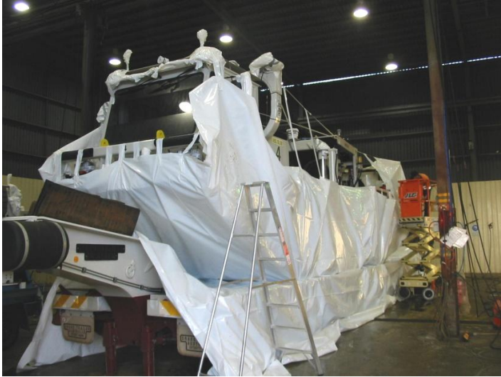
Attach Inner Base Sheet
