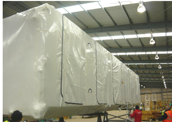
Outer Cover, Door Access Panels and Fumigation Panels Fitted
