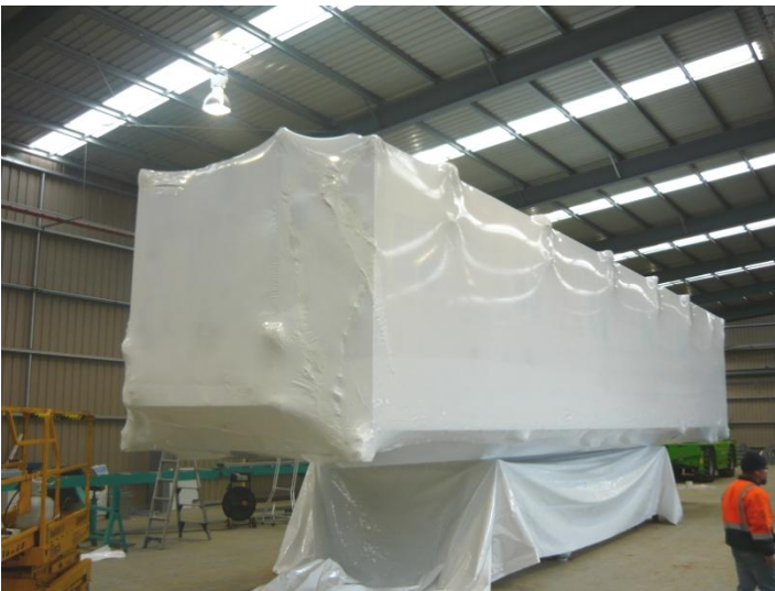
Inner Cover Fitted, Out Cover Next
